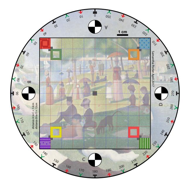
Photogrammetric Scale with cross non-coded markers PDF should be not be resized during printing (i.e. should be printed at 100%)
